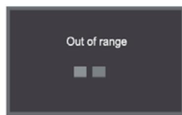
The monitor will be displayed out of range if the monitor exceeds the maximum resolution.
